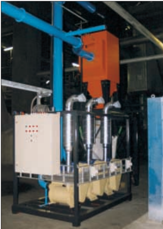
Several turbo-compressors applied in a Kiekens centralized vacuum system.
